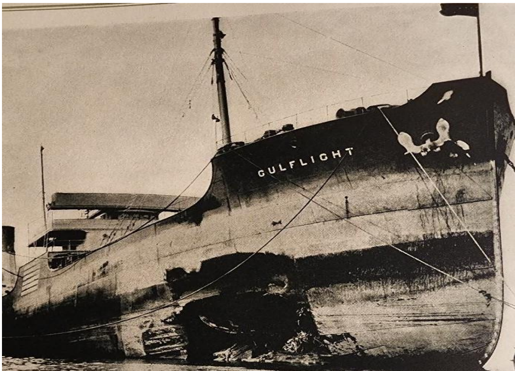
SS Gulflight in port showing the results of the torpedo damage
