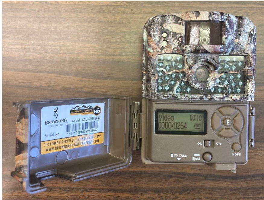
Figure 18. Interior features of the Browning Strike Force trail camera, including SD card storage capacity, delay time, and model number.
