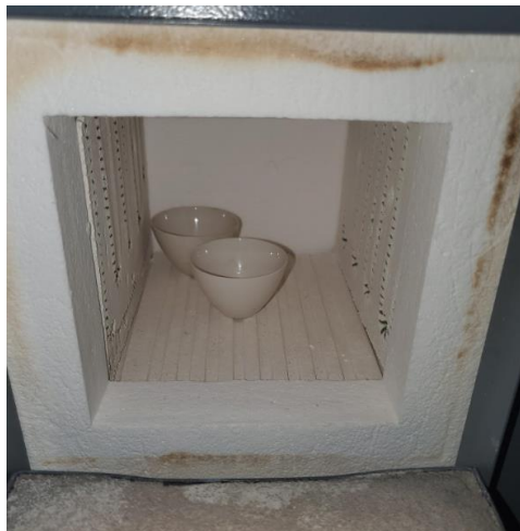
Image 13. Picture of oven set up for soil organic matter experiment.
