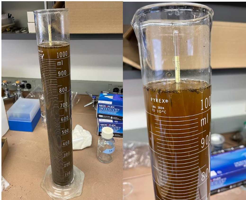
Image 11. Pictures of soil texture hydrometer method. The left image shows the state of the experiment after 40 seconds and the right image shows it after two hours.
