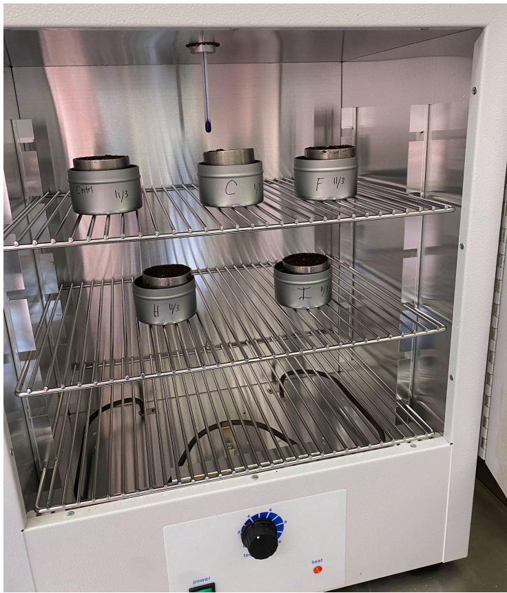
Figure 8. Soil cores in the oven as per the measurement of soil bulk density.
