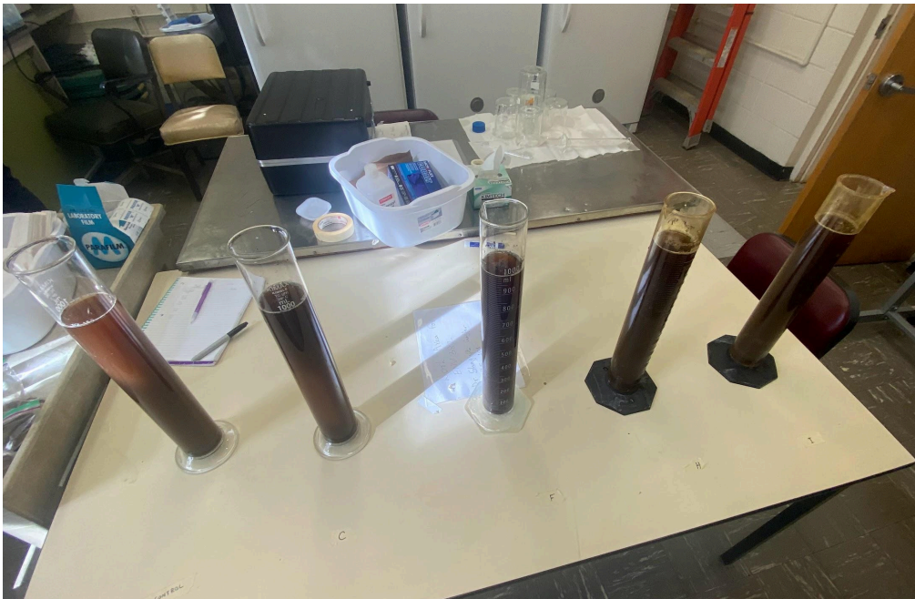
Figure 9. Hydrometer method lab setup.
