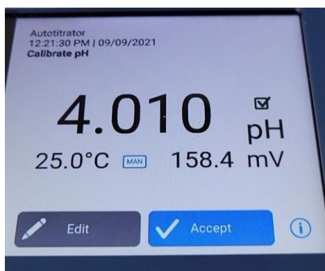
Figure 1. Example of the calibration screen. Note the checkmark next to the pH reading, indicating that the reading has settled on a number.
