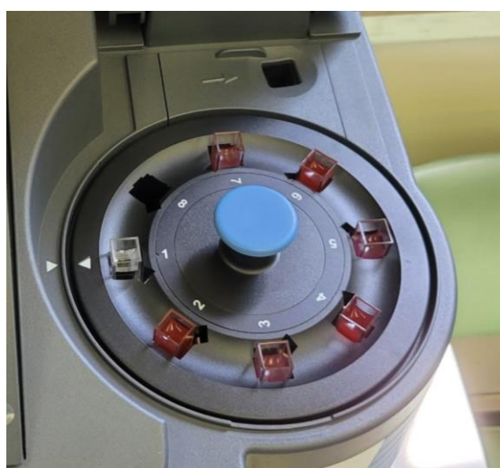
Figure 3. The cell changer on the spectrophotometer. Note the triangles on the cell changer and the machine. These triangles must line up before starting the run so the cell changer starts at slot 1.
