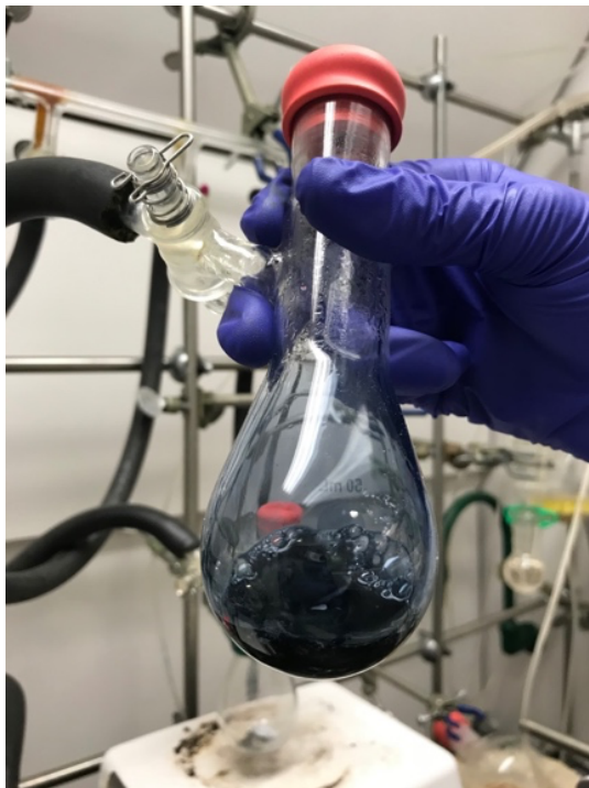
Figure 1.9: \text{SmI}_2 in THF. The completion of the synthesis is determined by the formation of the characteristic deep blue color.
