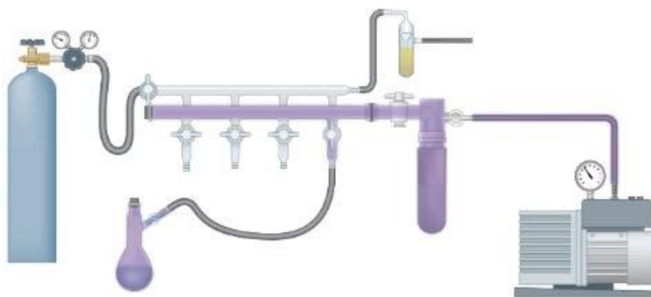
Figure 4: Graphic of a Schlenk line: glassware is attached via a hose and the flow of an inert gas or a vacuum is controlled by a valve
