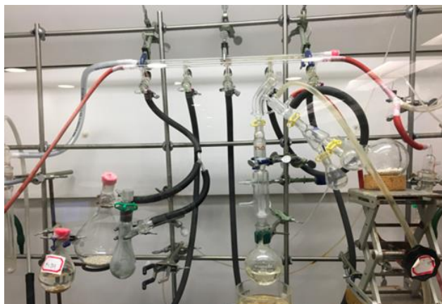
Figure 5: A Schlenk line which creates inert environments within the glassware through the steady flow of argon gas
