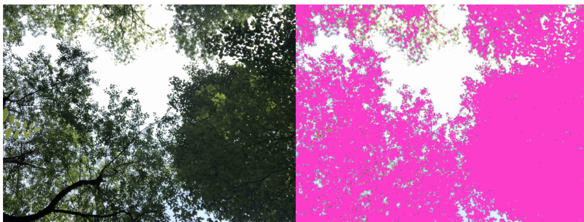
Figure 4. An image of the canopy taken above plot center (left) and the same image post-analysis in the mobile app CanopyApp (right). The app's software identifies and calculates the percentage of pixels in the picture that contain structures intercepting light, shown in pink.
