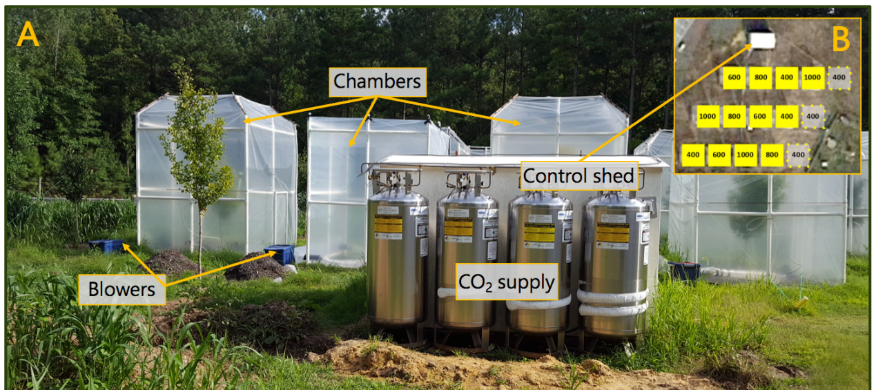
Figure 9. Experimental setup at the Smithsonian Environmental Research Center in Edgewater, Maryland. Trees are in open-topped chambers aside from outdoor control trees (pictured on the left). The control shed houses monitoring equipment as well as the supply of CO 2 . Blowers combine ambient air and CO 2 from the control shed into each of the chambers.
