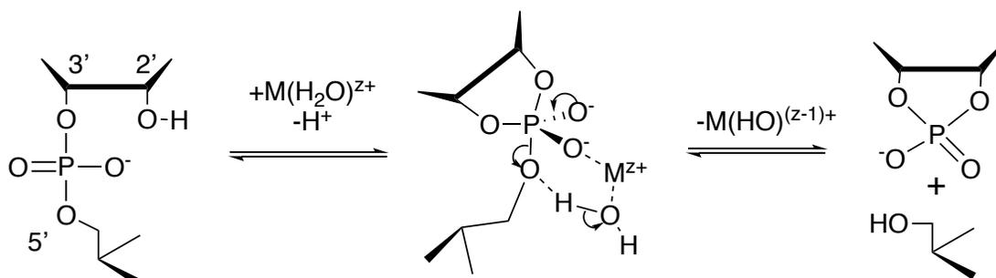
**Figure 6 Metal ion catalyzed hydrolysis of a phosphodiester in RNA with an internal Nucleophile.** Modified from Lönnberg et.al<sup>11</sup>. The cleavage of the RNA backbone is successful due to metal ion catalysis. The metal ion chelates to the non-bridging oxygen and activates a water molecule, to be used as an acid. The water molecule protonates the bridging oxygen, thus cleaving the phosphodiester.
