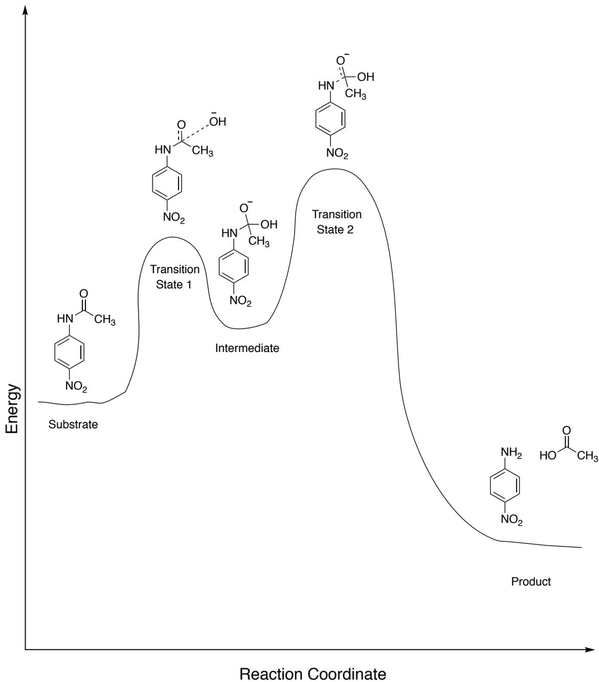
**Figure 24** Reaction coordinate of the hydrolysis of *p*-nitroacetanilide<sup>34</sup>. The hydrolysis of *p*-nitroacetanilide is believed to be done in a stepwise reaction, where there is a tetrahedral intermediate present. The rate-determining step is thought to be that of transition state 2 where the C—N bond is breaking.
