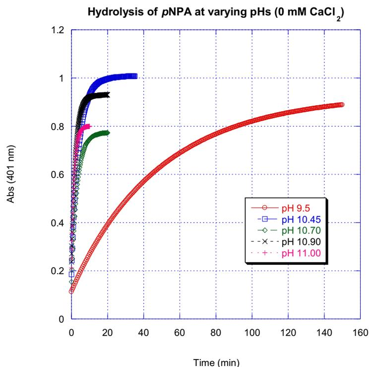
**Figure 27 Hydrolysis of *p*NPA at varying pHs with 0 mM [CaCl<sub>2</sub>].** These data were found using UV-Vis Spectrophotometry, measuring the appearance of the product, *p*-nitrophenolate at the absorbance, 401 nm. The reactions contained 50 mM of CAPs buffer, 0.05 mM of *p*NPA, 1000 mM NaCl at the varying pHs. The rate of hydrolysis increases as the pH is increased.
