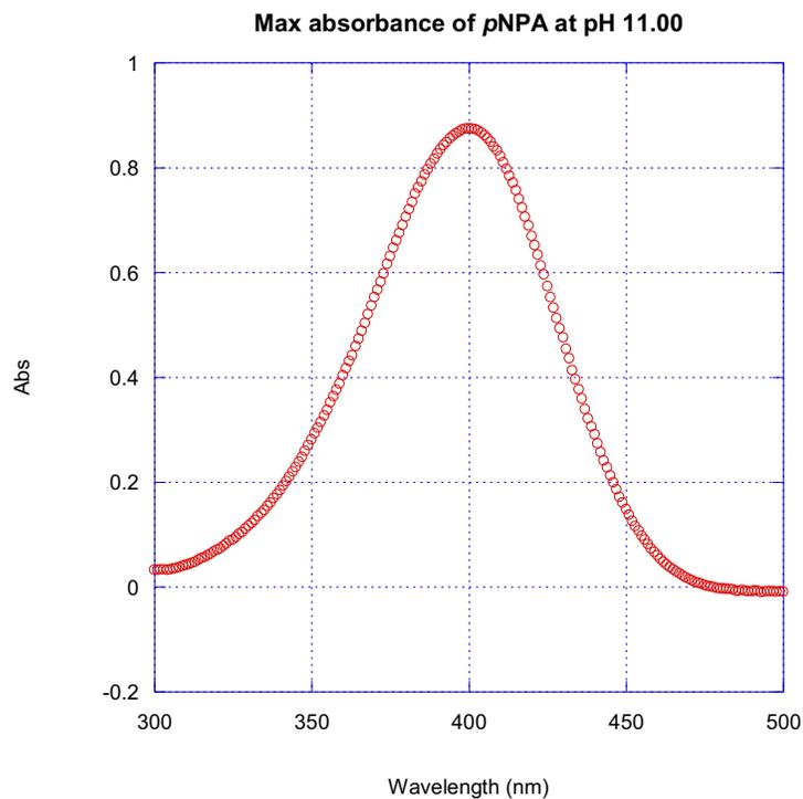
**Figure 26 Max absorbance of *p*NPA's hydrolysis product, *p*-nitrophenol.** Using UV-Vis Spectrophotometry, the hydrolysis product of *p*NPA, *p*-nitrophenol, at pH 11.00 was shown to have a  $\lambda_{\text{max}}$  of 401.0 nm.
