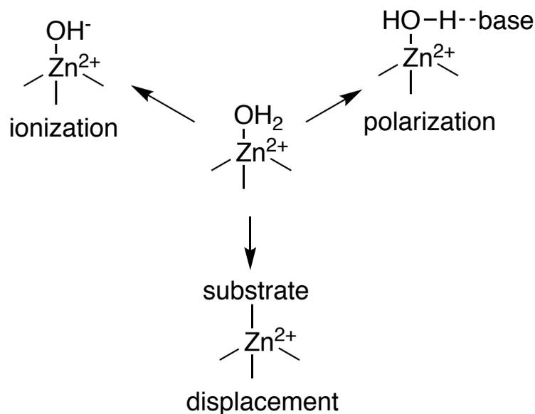
**Figure 2 Different functions that zinc-bound water can have.** The zinc-bound water can be ionized, polarized, or displaced by a substrate.
