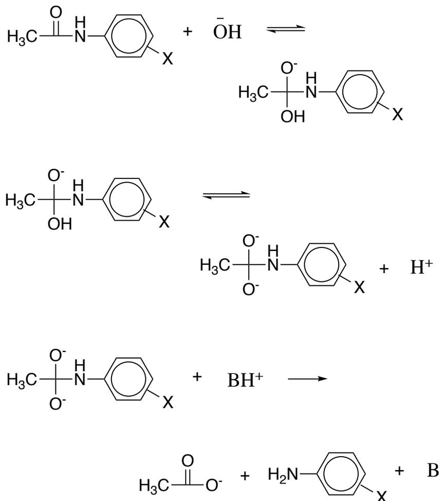
**Figure 23 Proposed mechanism of anilides with one hydroxide present<sup>32</sup>.** The previous anilides studied were found to utilize only one hydroxide ion. This hydroxide ion is used as a nucleophile to attack the carbonyl carbon to form the tetrahedral intermediate.
