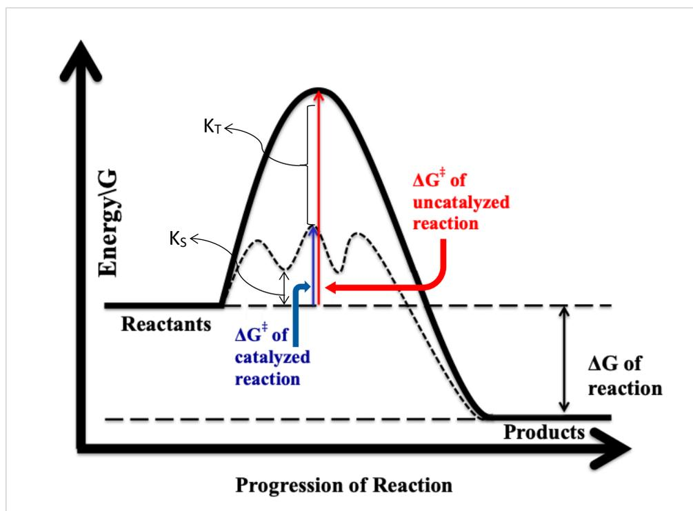
**Figure 1B Energy diagram of a non-catalyzed reaction versus a catalyzed one<sup>3</sup>.** The red arrow indicates the activation energy needed for an uncatalyzed reaction. The blue arrow indicates the activation energy needed for a catalyzed reaction to occur.
