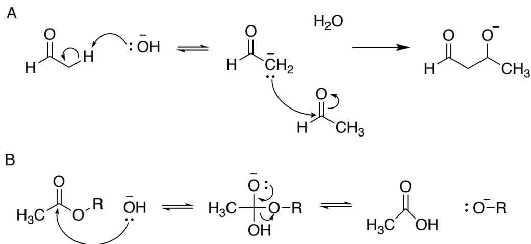
**Figure 12 Different ways that hydroxide ions catalyze reactions.** Two mechanisms in which hydroxide ions catalyze reactions. (A) A hydroxide ion is used to convert the substrate into its conjugate base and the conjugate base reacts. This particular reaction is an aldol reaction<sup>17</sup>. (B) A hydroxide ion combines with the substrate and the transition state contains the substrate and hydroxide ion.
