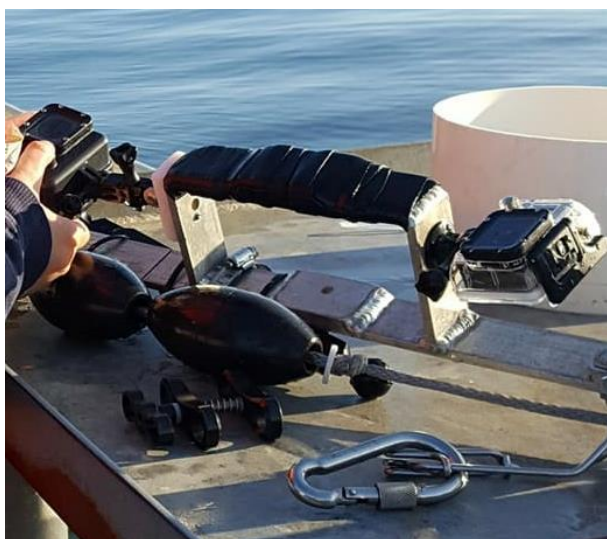
Fig. 4 The smaller adaptation of the BASS cam is equipped with two GoPro HERO4 Black Edition cameras encased in Sexton GoDeep Acrylic housing. Two Bigblue LED lights (72000 lm) illuminate the field-of-view at depth. This camera system is deployed vertically, with one end attached to a CTD wire and the other end attached to various weights.
