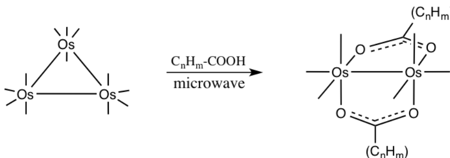
Figure 35 – Scheme of Powell's microwave-assisted reaction of \text{Os}_3(\text{CO})_{12} with carboxylic acids.
