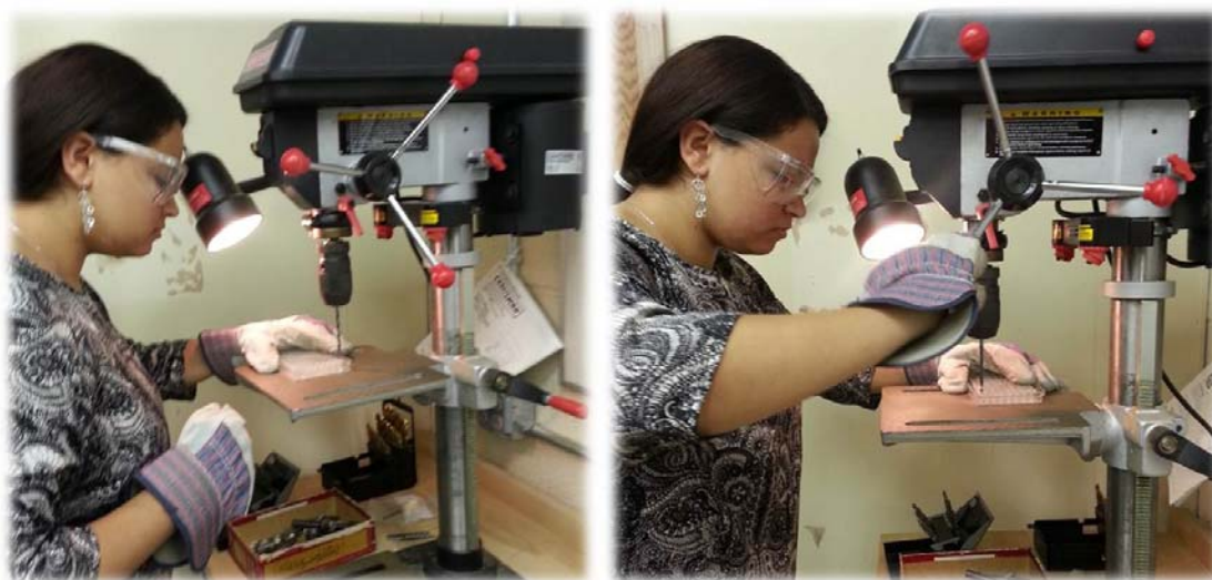
Figure 11: Attempt at creating improvised BBB mimicking apparatus. Here, holes are being drilled into the bottom of a 96 well plate to form a top plate onto which an artificial membrane can be placed. This apparatus failed due to the instability of the membrane on top of the hole in the plate.
