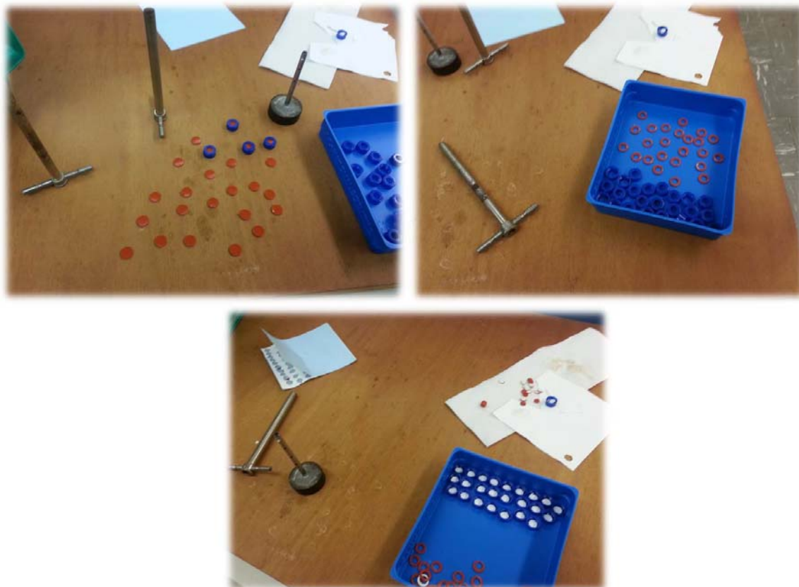
Figure 12: Another attempt at creating an improvised version of the BBB mimicking apparatus. This involved the replacement of rubber in the caps of 1 ml vials with the artificial membrane. The membrane was supposed to be held in place by a rubber gasket created out of bored rubber that was originally the cap of the vial. This apparatus failed due to leaks.
