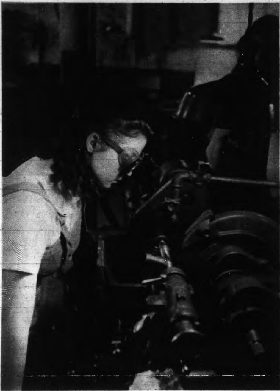
Machine Shop — Having turned it down on a lathe to its approximate size, Alice Williams precision-grinds a head stock spindle to the required final dimensions.
